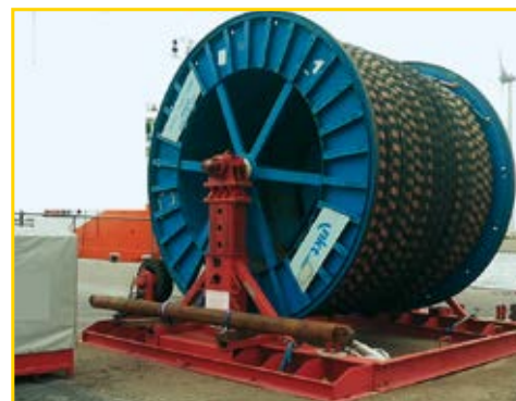
Kabel spoel machine 60T Cable Reel Stand 60T
