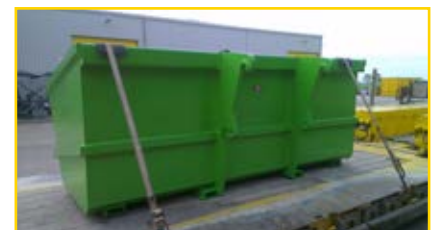
Afvalbak tbv wiellader Waste bin for front end loader
