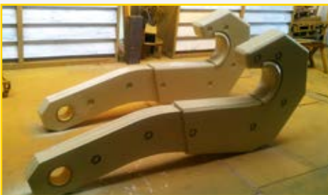
Lamellenhaken WLL 80T Laminated hooks WLL 80T
