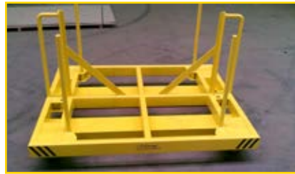
Transportkar ten behoeve van roosters Transport trolley for grates
