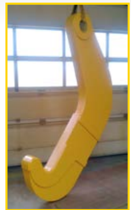
Hijshaak WLL-100T Lifting hook WLL-100T
