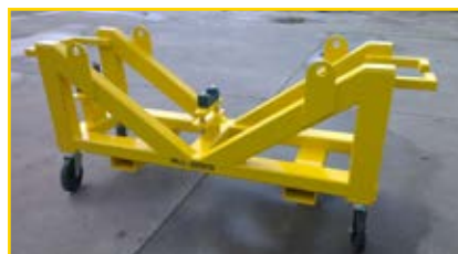
Transportkar turbine-as Turbine shaft transport trolley
